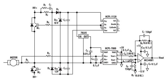
Figure 13. Motor Current Sensing Circuit
