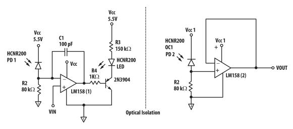
Figure 2. Positive Polarity Input Voltage Analog Isolation Amplifier Using the HCNR201 in Photo-Conductive Mode
