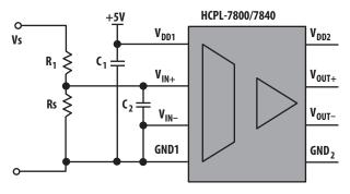
Figure 11. General Voltage Sensing Circuit
