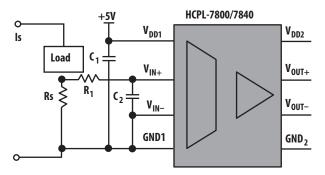
Figure 12. General Current Sensing Circuit
