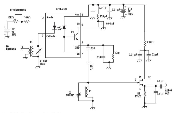
Figure 8. Optically Coupled Regenerative Audio Receiver
