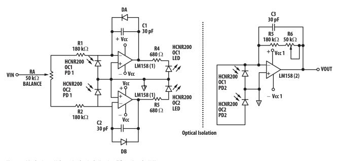
Figure 3. Bipolar Input Voltage Analog Isolation Amplifier using the HCR201
