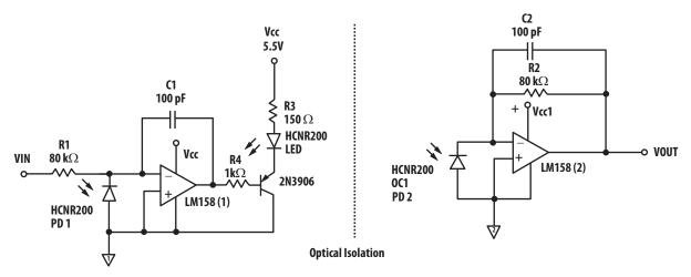
Figure 1. Positive Polarity Input Voltage Analog Isolation Amplifier using the HCNR201 in Photovoltaic Mode
