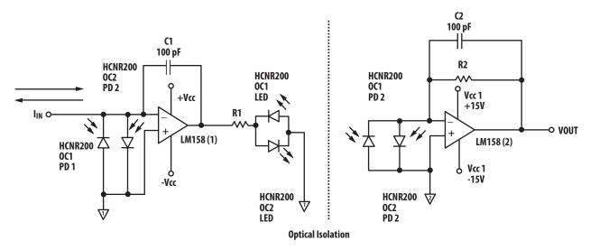
Figure 4. Current-to-Voltage Converter using the HCNR200
