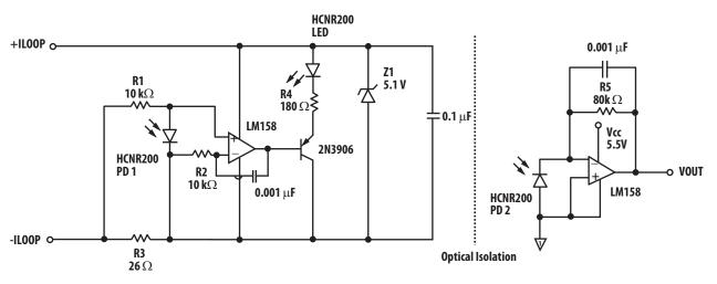
Figure 6. Isolated 4-to-20 mA Analog Receiver Circuit using the HCNR200
