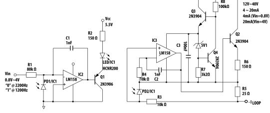
Figure 5. 4 to 20 mA HCNR200 transmitter circuit
