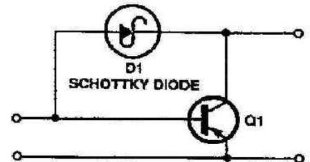
*Fig. 2 Schottky clamp diode used for improved switching speed.*
