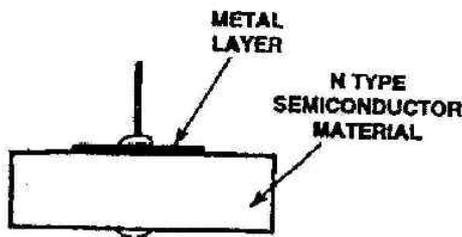
*Fig. 1. Basic construction of a Schottky diode.*
