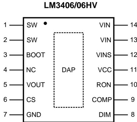
**Figure 1. 14-Lead Exposed Pad Plastic TSSOP Package
