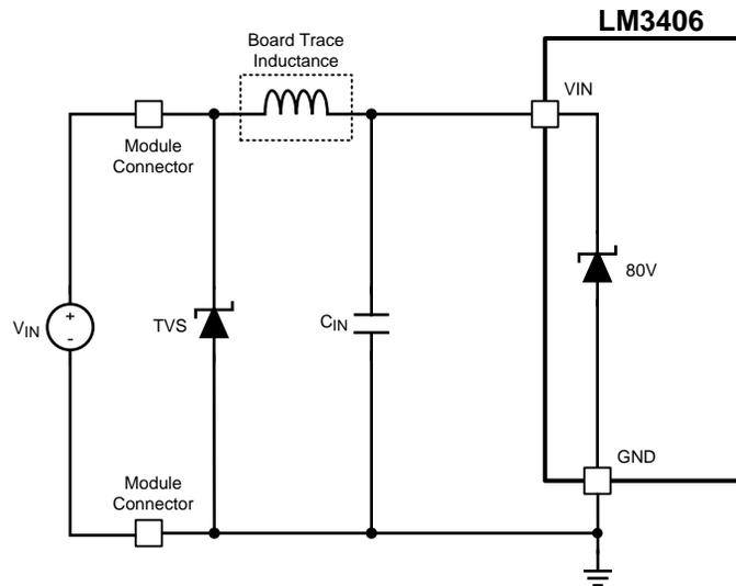
Figure 22. VIN Pin with Typical Input Protection
