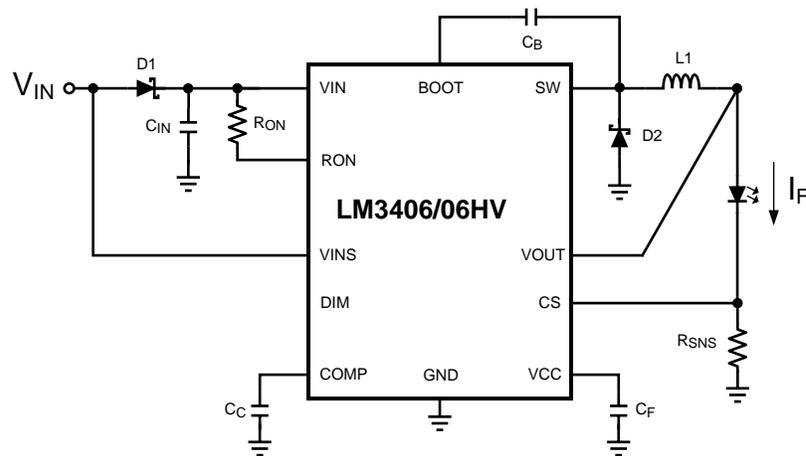
Figure 13. Typical Application using Two-Wire Dimming
