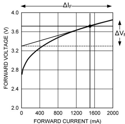
Figure 27. Calculating r<sub>D</sub> from the V<sub>F</sub> vs. I<sub>F</sub> Curve
