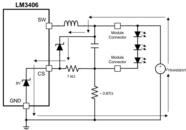
Figure 20. CS Pin with OVP, Transient Path
