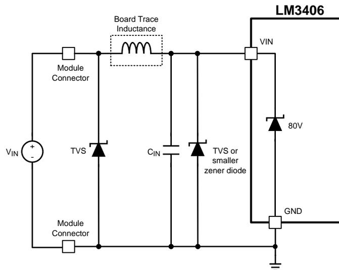
Figure 23. VIN Pin with Additional Input Protection
