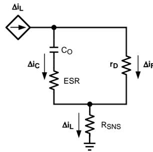
Figure 17. LED and C<sub>0</sub> Ripple Current
