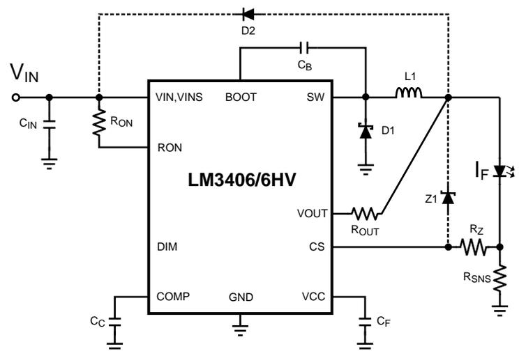
Figure 15. Two Methods of Output Open Circuit Protection
